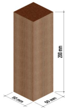
Fig. 2. Size of specimen compressive test.
